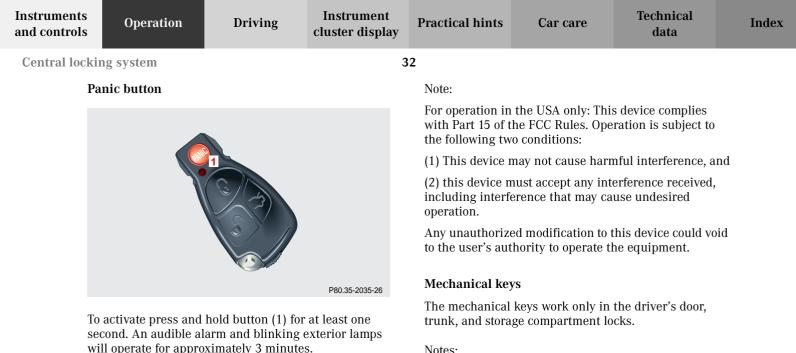
To deactivate press button (1) again, or insert electronic key in steering lock.
